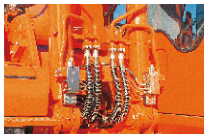
Boom and arm hose rupture protection valve
